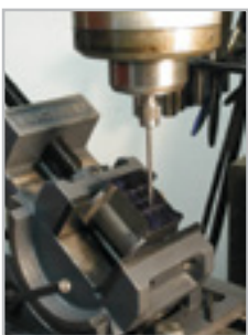
Needle Point shank being used to locate center on workpiece
