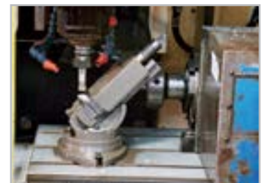
The Angular Machine Vice being used for 45° face milling
