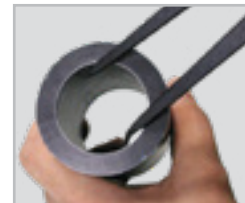
Inside Caliper: Used to measure the internal diameter of a cylinder
