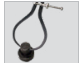
Outside Caliper: Used to inspect the external diameter of a machined component
