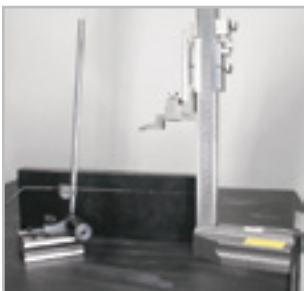
Surface Gauge being used to scribe a horizontal line parallel to the ground, on a work piece
