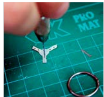
Pin Vice being used to hold a drill for hand-drilling on an electronic component
