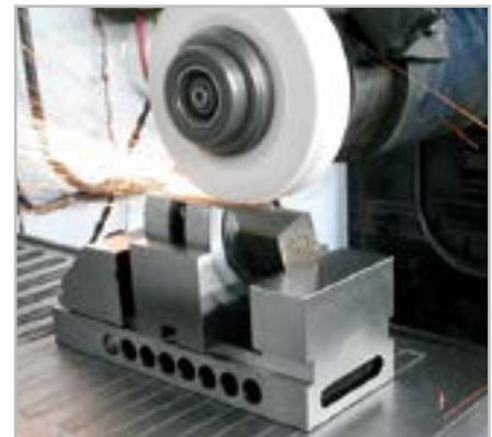
Toolmaker's Vice being used to hold a block of steel during grinding
