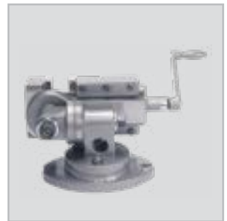
A typical case of the Universal vice set perpendicular to the base by rotation along the movable scale
