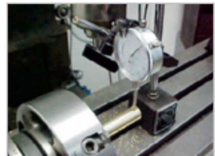
Magnetic base with dial gauge being used to check run out of a job on a lathe machine
