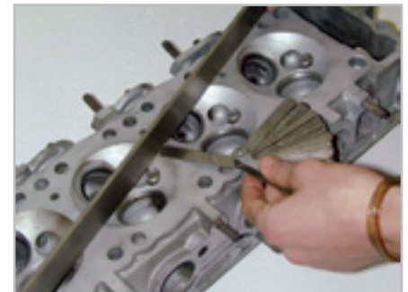
Straight Edge being used to check flatness of an engine block
