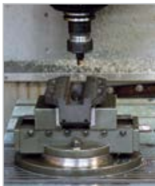
Self Centering Vice being used to mill key ways in the center of the casting
