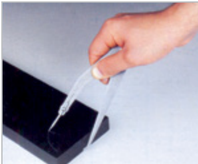
Jenny Caliper allows easy marking of arcs along the edge of workpiece
