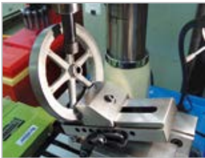
Sine Vice being used to drill an angled hole on a machine wheel
