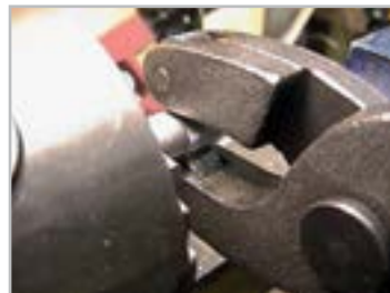
Knurling Tool Holder - being used for doing knurling on a job fitted onto a lathe machine
