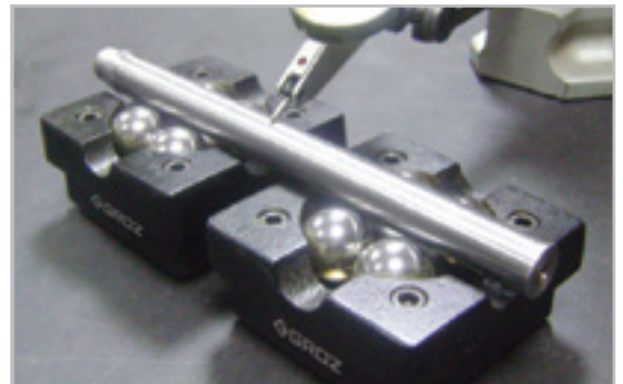
Ball bearing vee blocks with non-marring balls being used to check the roundness of a stepped rod
